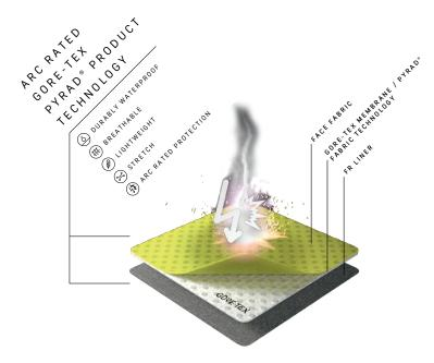
Material and garment construction are durably waterproof, windproof and highly breathable. Approved after rain tower test (EN 14360) new and after industrial laundry (ISO 15797, 60°C).
