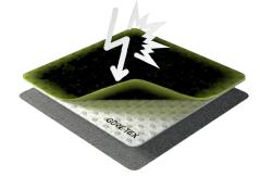
GORE-TEX PYRAD<sup>®</sup> fabric technology blocks convective heat flow during arc exposure and stops flame propagation by forming a carbonaceous char with the textile.
